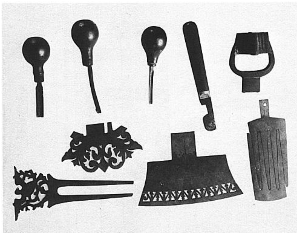
FIG. 6. SELECTION OF COMBMAKING TOOLS AND PATTERNS showing vidder and engraving tools. (Photograph courtesy of the Leominster Historical Society.)
